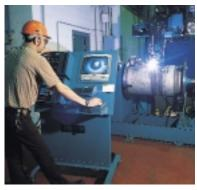
Columbiana's plasma welding capabilities assure that the internal welds of the cylinder will be precise and smooth. A smooth weld surface resists residue accumulation and facilitates cylinder cleaning. All welds are 100% radiographed.
