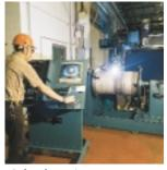
Columbiana's proprietary Plasma Smooth™ welding capabilities assure that the internal welds of a stainless steel tank will be precise and smooth. A smooth weld surface resists residue accumulation and facilitates tank cleaning.
