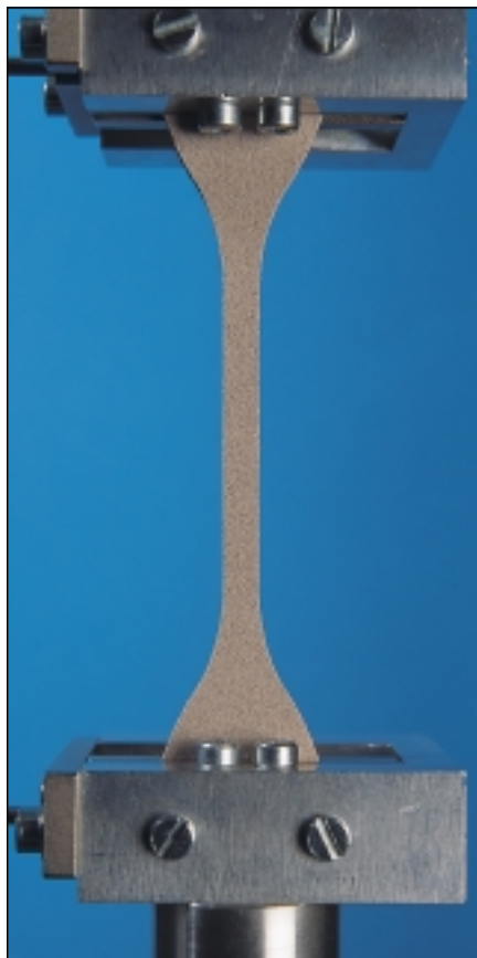
Stretch test demonstrating the superior strength and elasticity of T-form 400 gap filler. Elongations of up to 120% are achieved.
