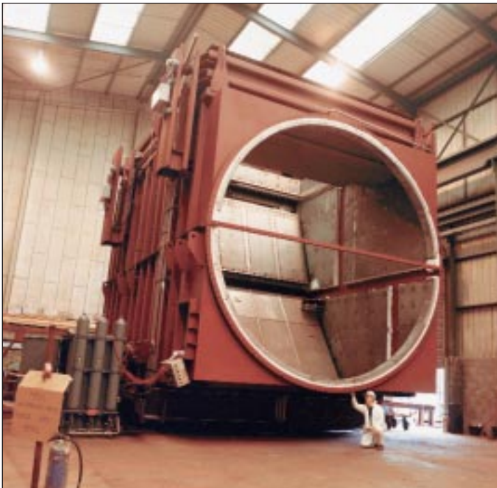
A triple blade diverter damper.
