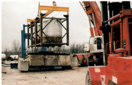
A prototype container design undergoing testing at Columbiana Texas. The in-house test facility permits Columbiana Texas to maintain full responsibility for container quality assurance. On-site testing also provides faster test results and shorter production times.
